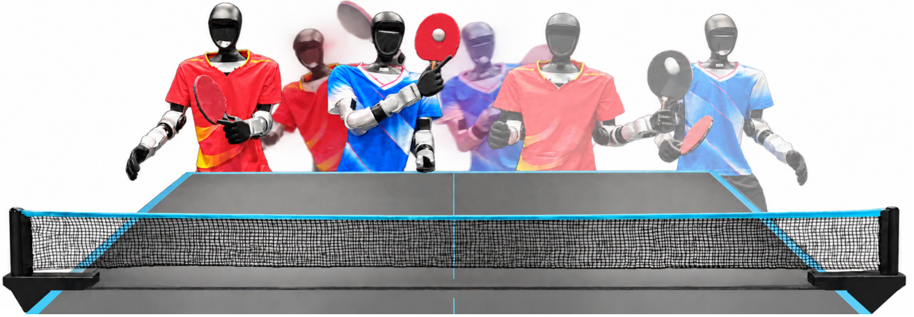
Fig. 1: PingpongDuo: the first table tennis doubles system on Humanoid. After returning a ball on the right side of the table, the red robot clears space as the blue robot moves left to receive the next ball, achieving the complete movement within one second.
